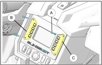
Align the screw holes of new colored media bezels
