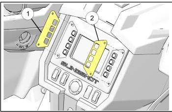
4. Fasten the colored media bezels ① and ② to infotainment center by using the four screws (A) removed in Step 2.
