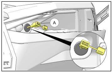
Access two bezel mounting screws
