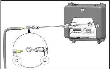
Reinstall touchscreen infotainment assembly (E), bezel (D), two bezel mounting screws (B), and USB port (A) removed in Touchscreen Infotainment Removal section.
