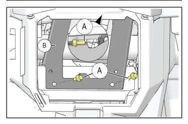
2. Install amp ③ to amp mounting bracket ⑧ with three screws ⑤.
