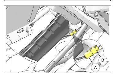
Use cable tie (6) to secure cables to vehicle frame.
