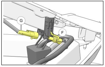
b. Connect antenna connector ⊕ to brake light connector ⑥. Connect electrical harness connector ⊕ to antenna connector ①.
