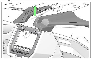
4. Remove two bezel mounting screws
