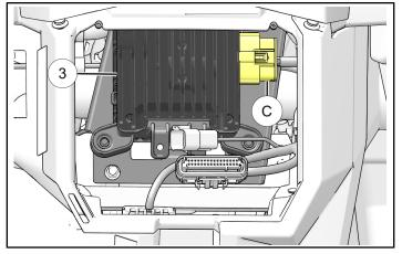
5. Connect antenna harness connector 0 to touchscreen infotainment connector E.
