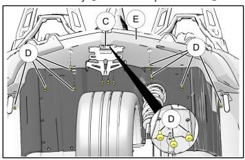
3. Install antenna ① onto top side of antenna mount bracket as shown.
