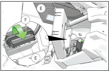
6. Remove touchscreen infotainment assembly from dashboard and carefully place assembly where it will not be damaged.
