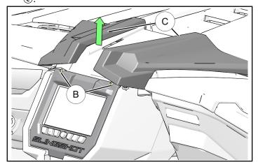
4. Remove two bezel mounting screws ® and bezel ®.
