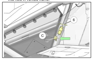
3. Install speaker assembly ② to vehicle frame with three screws ④.
