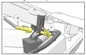
b. Connect antenna connector (f) to brake light connector (g). Connect electrical harness connector (F) to antenna connector (J).
