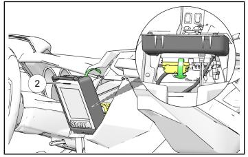
Install bezel (5) with two bezel mounting screws (A) retained from Step 2 of Removing Stock Parts section.
