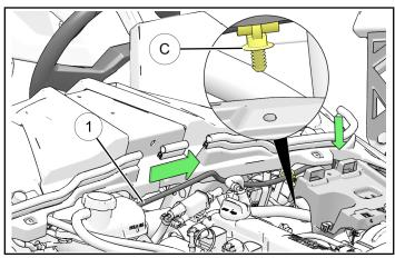
3. Continue to route radio harness ① towards outside of vehicle frame and under outside frame joint using harness cable tie ⓒ and cable tie ⑨ to attach radio harness ① to frame.
