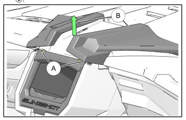
2. Remove and retain two bezel mounting screws (A) for **Touchscreen Infotainment Installation section**.
