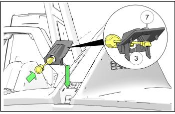
5. Remove electrical harness connector cover from electrical harness connector (f) and connect camera harness connector (f) to electrical harness connector (f).
