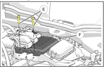
b. Slide ECM mount (F) with electrical harness attached away from chassis mount (G) towards front of vehicle and gently place out of way.
