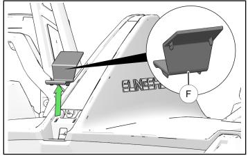
Install rear camera ③ into rear camera mount ⑦ and press unit securely into place where discarded trim (F) was removed from.
