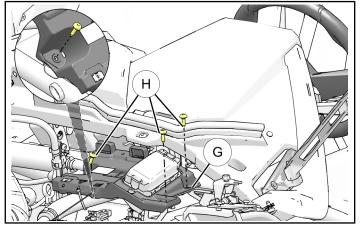
d. Tilt chassis mount (c) slightly to access hole that push pin rivet will be installed into.
