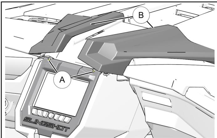
2. Remove two bezel mounting screws (A) and bezel (C).
