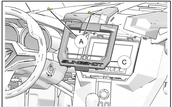
3. Tilt touchscreen infotainment assembly ① forward and pull assembly out with electrical harness still attached. Rest touchscreen infotainment assembly ① carefully on center console where it will not be damaged.
