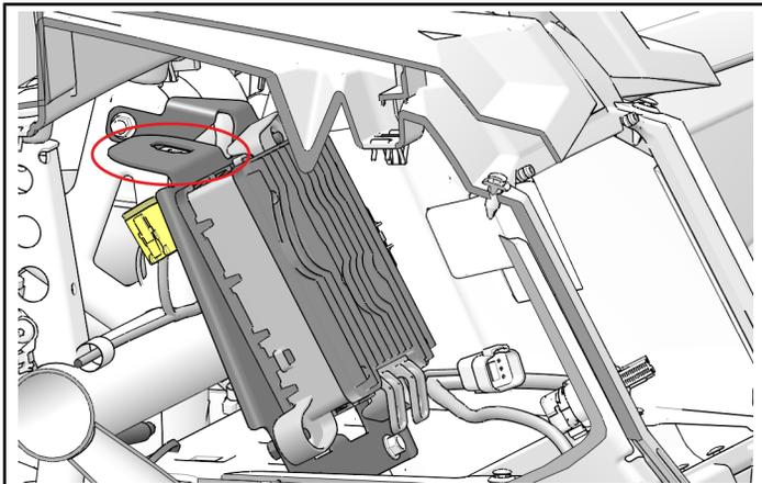
2. Remove protective backing from adhesive tape and firmly mount GPS ① with embossed arrow pointing towards front of vehicle.
