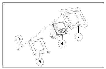
Position PMX assembly at edge of dashboard cavity. Join antenna harness connector 5C and power connector 3D to rear of PMX audio. Tilt assembly into dashboard until top snaps into place.
