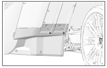
2. Remove two panel fasteners from battery access cover.
