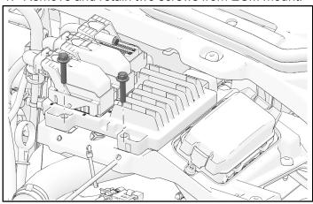
2. Slide ECM mount towards front of vehicle, with electrical harnesses still attached.
