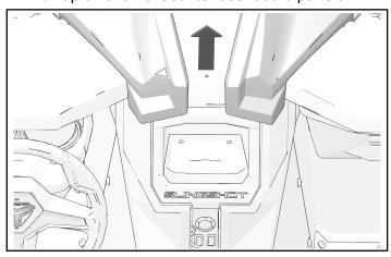
2. Remove bezel and two bezel fasteners.
