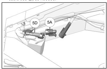
4. Route antenna harness through battery compartment toward front of vehicle along transmission tunnel. Secure with cable ties ®, as needed.
