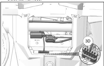
2. Route speaker connectors left and right along chassis, beneath front of dashboard.
