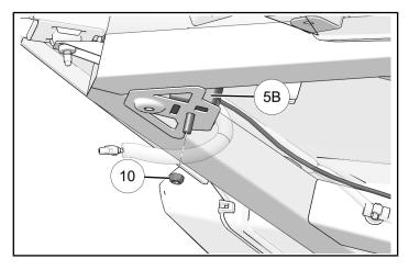
3. Join connector 5D to chassis electrical harness and connector 5A to brake light. Route antenna harness ⑤ to battery compartment. Secure with cable ties ⑧, as needed.
