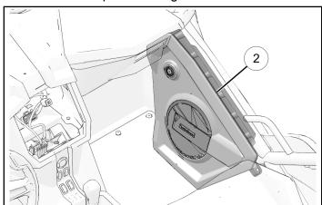
2. Join audio harness connector 3A to right speaker. Secure harness to vehicle with routing clip 3G and one cable tie (8).
