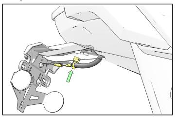
2. Install two push-pin rivets to complete battery cover installation.
