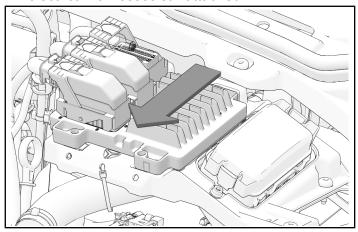
3. Remove and retain three screws from chassis mount. Cut cable tie to remove chassis mount from vehicle.
