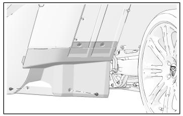
3. Slide battery access cover down-and-back to remove.
