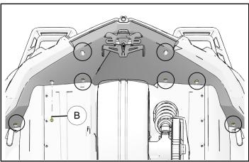
4. Ensure license plate light harness passes through underside rear deck while removing panel from vehicle.
