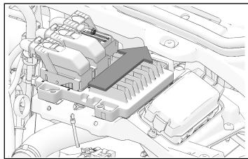
3. Install ECM mount with two ECM mount fasteners.
