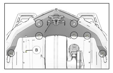
Connect license plate to license plate light chassis harness. Secure license plate light chassis harness to license plate mount with edge routing clip.
