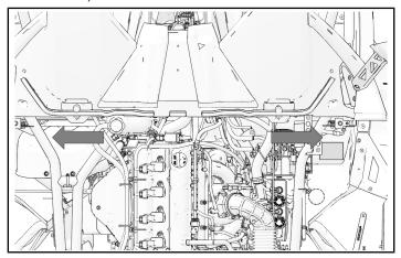
3. Secure left side of harness to ECM mount with one routing clip 3G. Route left-hand speaker connector 3A down to driver-side floor board.
