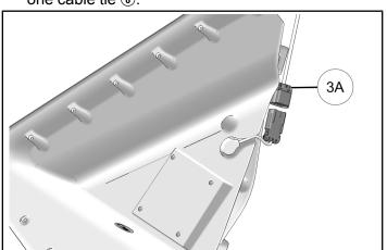
3. Install speaker to vehicle with three speaker fasteners ①.
