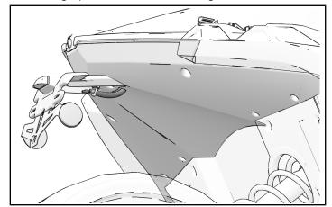
2. Begin securing underside rear deck panel with one screw (A).
