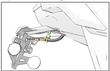
2. Remove and retain one screw (A) from underside of license plate mount assembly.
