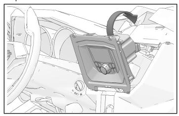
3. Install bezel over PMX audio with two retained bezel fasteners.
