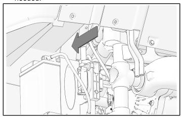
5. Remove two cup holders to access transmission tunnel.
