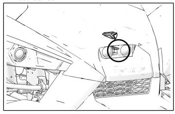
2. Firmly pull hood handle upward and forward, rotating hood to vertical position in front of vehicle.
