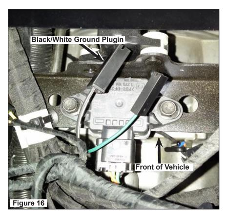
9. Reinstall ECU bracket, unit and center console (or radio) according to service manual and the reverse of steps (3, 2, 1) from mounting preparation.
