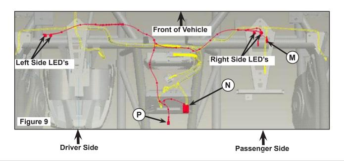
2. Feed the wire harness without the power terminal, as shown in Figure 10, starting from inside the console. Feed left side wires and LED's left out into the engine area, along the existing wiring to the drilled holes, as shown in Figure 11.
