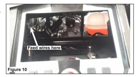
3. Feed left LED wires along the existing wiring harness, according to Figure 9, zip tying wiring approximately in the areas indicated in Figures 11a, 11b, and 11c.
