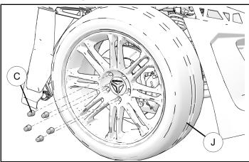
3. Carefully remove driver side front wheel (J) from wheel mounting bolts and set aside.
