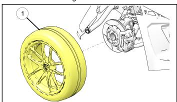
5. Hand tighten five lug nuts ⑤, ensuring the wheel hub face is mated to the bearing hub face. Torque lug nuts ⑤ to specification in a star pattern.
