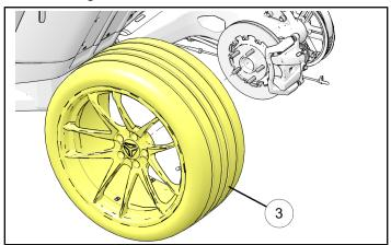
4. Hand tighten five lug nuts ⑤, ensuring the wheel hub face is mated to the axle hub face. Torque lug nuts ⑤ to specification in a star pattern.
