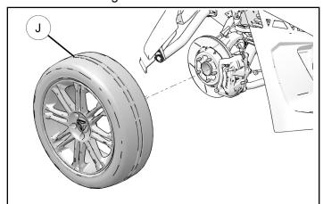
4. Check the directional arrows on the tire to ensure the correct placement of the front wheel assembly
