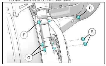
2. Use floor lift to slowly lift rear of the vehicle. Continuously check clevis bolts, at certain height all bolts will become loose. Leave floor jack at this height and remove three bolts (F) and (G). Retain fasteners for re-installation.
