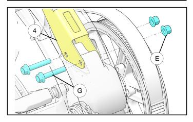
Install clevis (4) to rear shock at the top using bolt (F) and nut (D). Torque bolt to specification. This joint should be torqued under a lightly loaded state to account for clearances.
