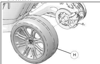
3. Place rear wheel assembly ③ onto the wheel mounting bolts.
