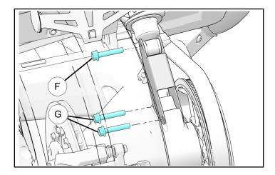
3. Position the premium lower shock clevis ④ onto the swingarm and install two bolts (G) and nuts (E) using 15mm wrench. Torque bolts to specification using torque wrench.
