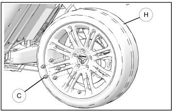
2. Carefully remove rear wheel (H) from wheel bolts and set aside.
