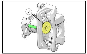
5. Once the piston has been pushed in far enough, re-install the brake pads (G) and (H) and calipers and move on to Step 13 of Instillation section.
