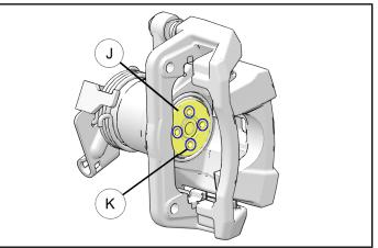
3. In order to push the piston (J) back, use a special disc brake piston tool. If disc brake piston tool is not available, needle nose pliers works as well.
