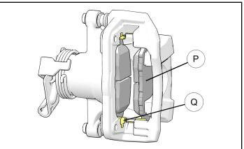
10. Install new brake pads (2) by first installing new springs (R) and then placing pads within springs.
