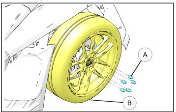
5. Remove wheel (B) from the wheel mounting bolts (C).
