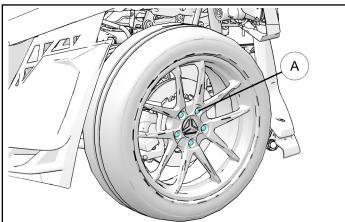
3. Using floor lift slightly raise passenger side of vehicle off the ground. Refer to "Lift Placement" section on last page of the instructions.
