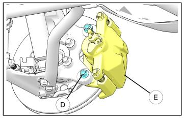
NOTE When removing caliper, use care not to damage brake line. Support caliper to avoid kinking or bending brake line.
