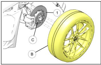
14. Reinstall lug nuts (A) removed in Step 4 to hold wheel in place. Use torque wrench to tighten nuts (A) to specification.
