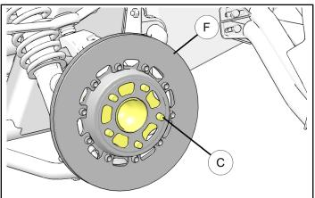
8. Install new rotor assembly ① onto wheel bolts (C).
