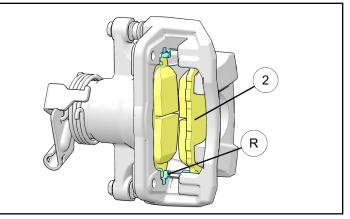
Install caliper (E) on the rotor assembly ①. If brake pads do not fit around new rotor, see "Brake Piston Adjustment" section. Once pads are around rotor, install upper and lower caliper mounting bolts (D) removed in Step 6. Using torque wrench, tighten caliper bolts (D) to specification.
