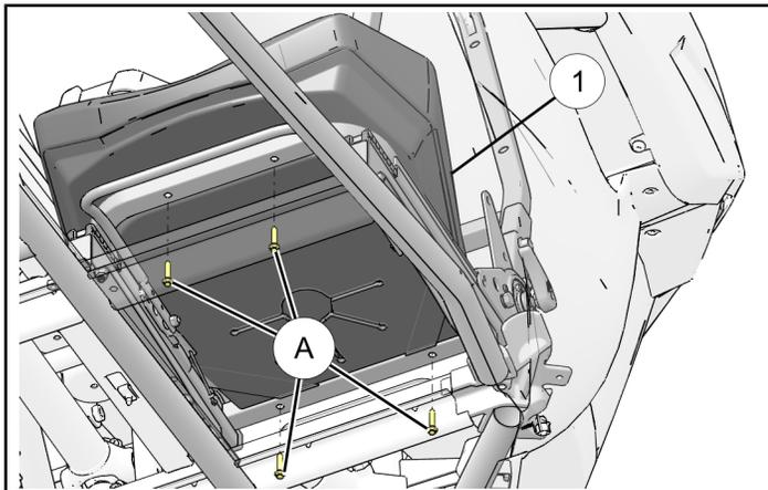
3. Position top of seat forward and install upper cushion ② by first sliding headrest on to bracket and then firmly pushing back.
