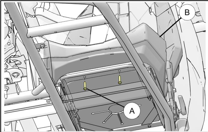
3. Position driver seat all the way forward and rotate top part of seat forward. Remove and retain two screws **A** located at back of bottom cushion.
