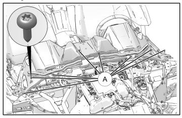
3. Torque eight screws to specification.
