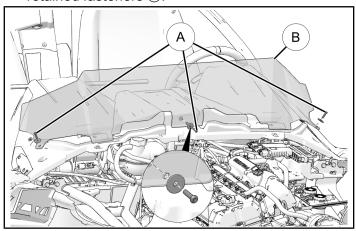
2. Torque fasteners to specification (if applicable).
