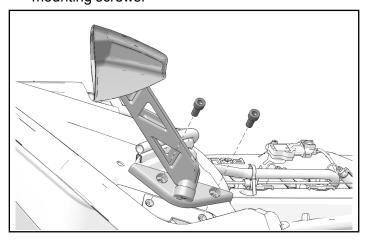
2. Torque mounting screws to specification.
