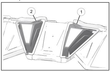
2. Open bags and mark hole locations on dashboard with a light colored marking device.
