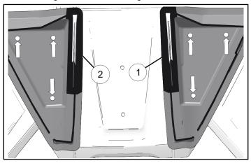
3. Drill six 11/32 in (8.5 mm) holes in center of marked locations.
