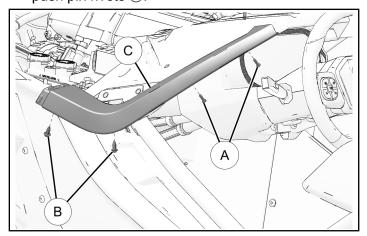
2. Torque two screws to specification.
