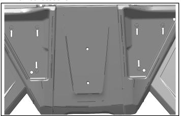
4. Set bags in place and install six push rivets ③ into holes
