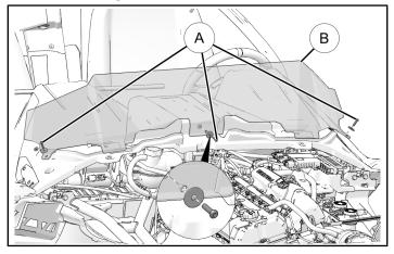
2. If equipped, remove and keep screw, washer and O-ring from center windshield mount.
