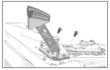
2. Torque mounting screws to specification.
