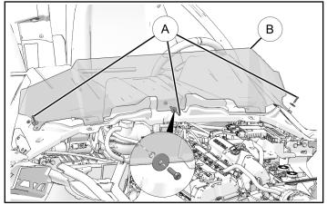
2. Torque fasteners to specification (if applicable).
