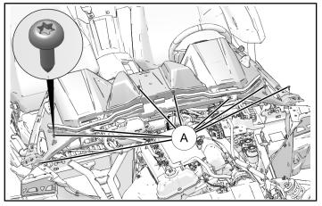
3. Torque eight screws to specification.
