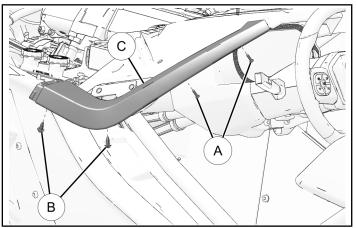
2. Torque two screws to specification.
