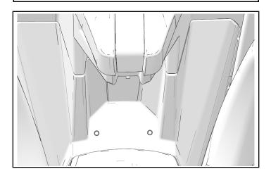
6. Remove and keep two screws (A) from center console opening as shown.
