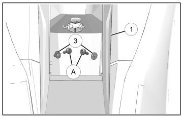
10. Align lower holes and install two push pin rivets ② into holes.
