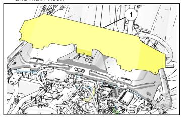
5. Mark location of center hole in front of windshield with a marker/pencil. Remove windshield from vehicle. Drill 1/2 inch hole in marked area. Insert third wellnut ② into new hole.
