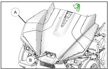
3. Press two wellnuts ② into driver and passenger side main visor panel holes ⓒ as shown.
