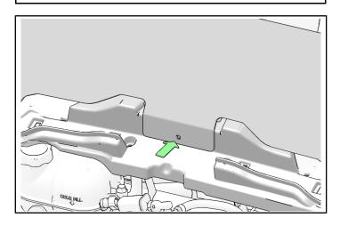
6. Reinstall windshield ① by engaging tab and slot in front and aligning three holes on windshield. Install screw ③ and washer ④ onto windshield. Torque screws to specification.
