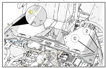
4. Install windscreen ① by first engaging tab and slot in front then align mounting holes on windshield and main visor.
