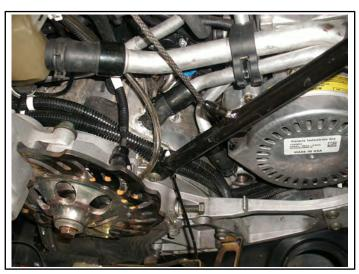
20. Install red cables ⑦ and ⑨ on to the solenoid with locking nut ⑪ and slide rubber protectors over solenoid nuts. Connect wiring harness ⑥ as shown. Torque the locking nuts ④ to below specification.
