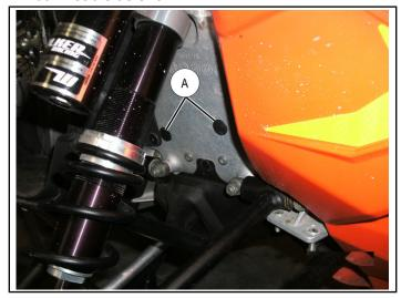
12. Install electric start bracket ③ to right side of the bulkhead using two screws ⑤ as shown, with T-30 torx. Torque bolts to specification.
