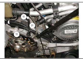
Install routing clip 3 into hole in battery box bracket and tie both red and black battery cable as shown.
