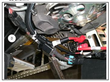
23. Install battery (E) (PN 4013045) and terminals as shown. Slide protective cover over the red terminal. Install battery box heat shield (6) and rubber strap (7) with D-rings (4) on the ends. Torque screw to specification.
