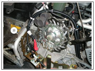
22. Install red cables (3) and (2) on to the solenoid with locking nut (30), and torque to specification.
