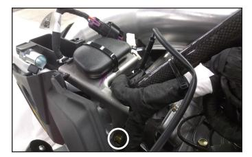
8. Connect GPS harness to vehicle diagnostic connector (J) as shown in figure. Install the diagnostic connector dust cap onto new GPS/ diagnostic cable connector.
