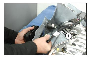
3. Connect key switch connector to harness as shown in figure.
