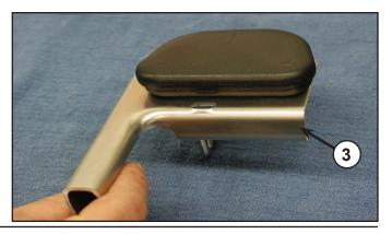
3. Using Panduit strap (4) supplied in the kit, install GPS antenna receiever on bracket and tighten.
