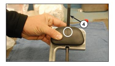
7. Install GPS assembly onto the vehicle at two mounting locations as shown in figures.
