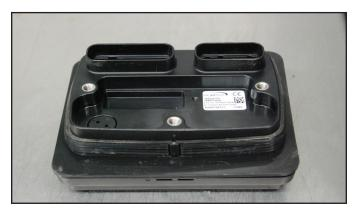
2. Install display gauge and hood harness (1) onto the vehicle hood. Connect display harness to PIDD as shown in figure.
