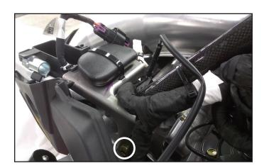
8. Connect GPS harness to vehicle diagnostic connector (J) as shown in figure. Install the diagnostic connector dust cap onto new GPS/ diagnostic cable connector.
