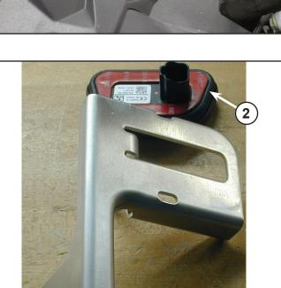
3. Using Panduit strap (4) supplied in the kit, install GPS antenna receiever on bracket and tighten.
