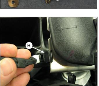
7. Install GPS assembly onto the vehicle at two mounting locations as shown in figures.
