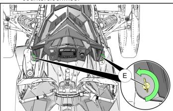
Slightly lift the rear of the hood assembly to gain access to the main hood harness connector ① and disconnect from main chassis harness connector ③. Cut the cable tie ④ securing the hood harness to the chassis and remove hood.
