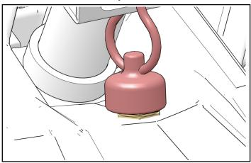
b. Start vehicle and remove tether cord to ensure it is functioning properly. Vehicle should stop running once tether cord is removed.
