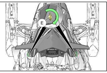
b. After installing hood, install both side panels making sure all latches and rubber straps are fully secured.
