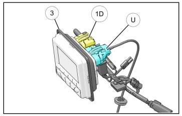
c. Connect the USB harness (1) that came with the PIDD 2.0 Kit (PN 2881554) to the corresponding port on the back of the digital display as shown.
