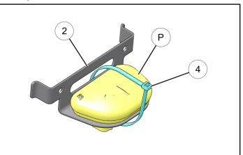
f. Place mounting bracket ② with GPS puck into position on the back side of the PIDD as shown and secure with provided fasteners ⑤. Tighten until snug being sure not to overtighten.
