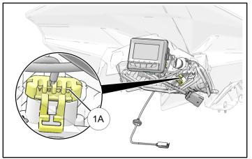
j. Cable tie remaining portion of the USB cable to the PIDD harness. Be sure to leave the USB connection readily accessible for use when updating the PIDD software. Refer to your PIDD user manual for details.
