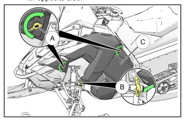
Next, remove the hood assembly D by first rotating the two hood latch fasteners E 180° counterclockwise.
