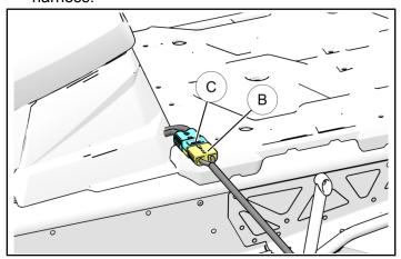
3. Next, remove protective cap ① from the winch power connection.
