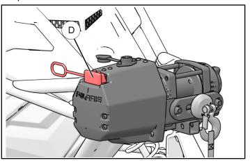
4. Route the front jumper harness around the left side of the vehicle and connect the remaining power connector (£) on the jumper harness to the winch power connection (£).
