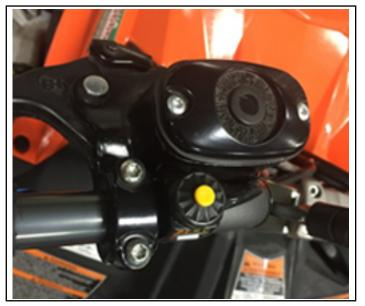
17. Assemble PERC engagement button (F) with a Phillips screwdriver back onto handlebars. Torque fasteners to specification.
