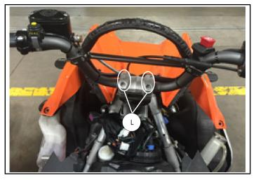
13. Follow hand warmer wires into handlebar harness cluster located next to steering column in front of fuel tank to unplug handlebar connection and remove connection and wires from harness cluster.
