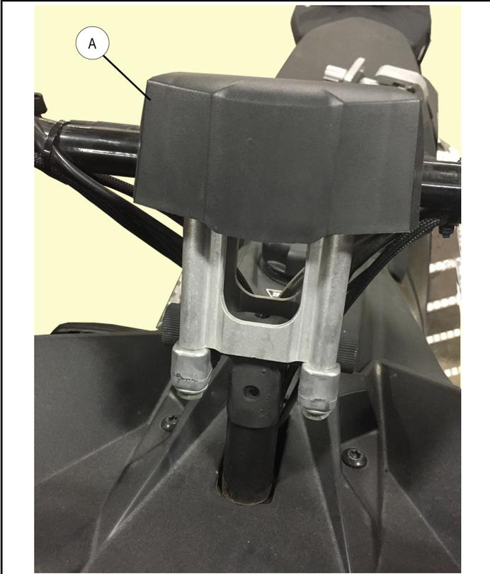
2. Remove four upper handlebar mounting bolts (B) and gently move handlebar assembly forward.
