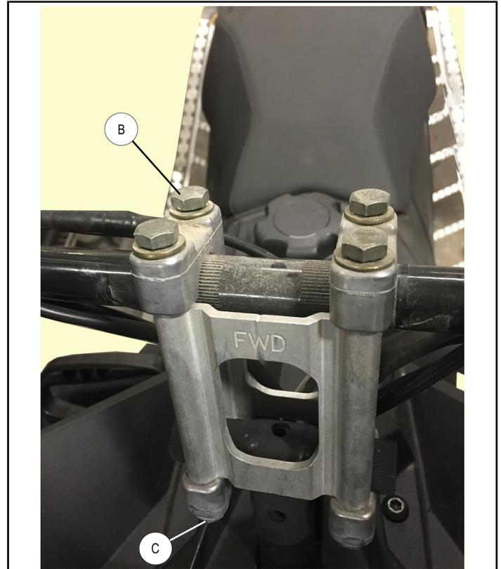
3. Install ROX handlebar riser ① on steering post with ROX riser cap ③ and mounting screws ④.
