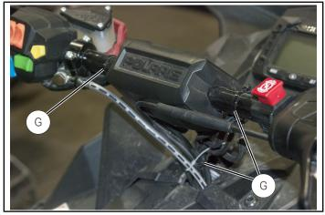
7. Remove the handlebar cover (AG).
