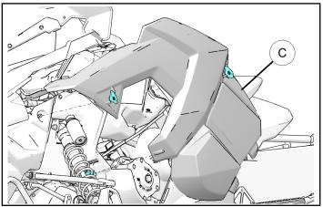
3. Rotate the 1/4 turn fasteners (D) at the rear corners of the hood (E).
