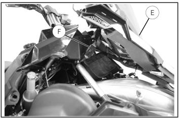
5. Remove the hood assembly (E) from the vehicle.
