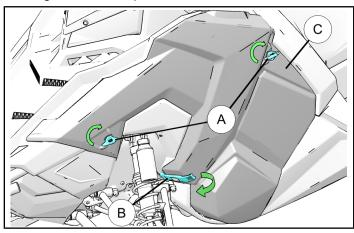
2. Open the side panel (C), then pull the panel outward to release the tabs at the bottom. Repeat the same for removing side panel on other side of vehicle.
