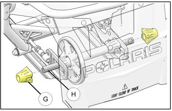
Remove axle shaft (H) holding inner black plastic spacers (M), bushings (L), center wheel (E), and spacer (K) in place on side rails (J). Discard bushings (L) and spacer (K). Retain all other parts for installation of new wheels.
