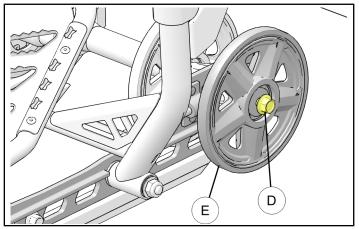
Remove rear axle bolt (D), washer (F), and outer axle wheel (E). Discard the bolt (D) and washer (F). New hardware is provided in the kit for installation. Repeat the same on other side of sled.
