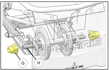
Loosely install new outer wheel ① onto the shaft (H) using bolt ③ and spring washer ⑤. Don't tighten the bolt ③. Repeat the same on other side of sled.
