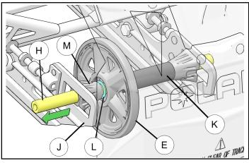
7. Insert axle shaft (H) from either side of rails (J) and install original inner black plastic spacers (M), new bushings ④, new inner wheels ①, and new spacer
