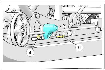
3. Place the wheel ① onto the wheel mount with the snap ring facing out as shown.
