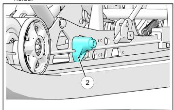
2. Next, insert the lower wheel mount bolt **6** from the outside as shown and fasten with the supplied locking nut **4**). Torque to specification.
