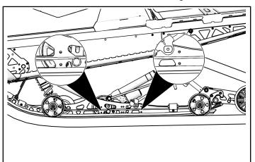
1. Place the wheel mount ② into the mounting location shown below and align with the mounting holes.
