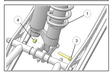
5. Install shock assembly ① onto rear torque arm using screw ③ and nut ④. Torque to specification.
