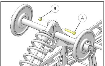
3. Remove screw (A) and nut (B) securing shock to the lower mount.
