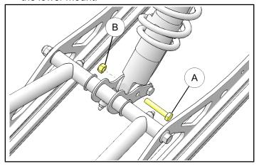
4. Install new shock assembly ① onto lower mount using screw ③ and nut ④. Torque to specification.
