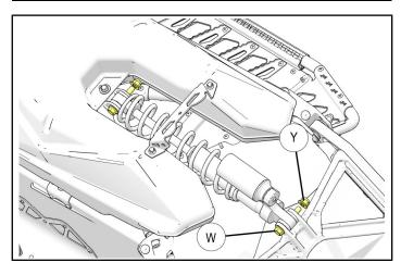
4. With the fuel tank still raised and moved slightly to the right, place the Fox air hose bracket ⑤ on left side of tunnel as shown. Using the bracket as a template mark and drill two 3/16" holes in the top of the tunnel. Using supplied rivets, rivet ⑪ the bracket ⑤ to the tunnel as shown below.
