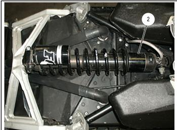
6. Install air fill assembly in bracket that was previously installed on tunnel and tighten lock nut as shown.
