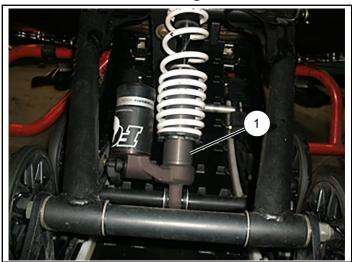
12. Once lower shock mounting components are accurately reassembled and aligned within rails. Use new screws (9) from kit to fasten back onto rails. Note there is a washer (N) that needs to be placed onto each screw. Ensure the Fox shock reservoir is orientated properly as shown above.
