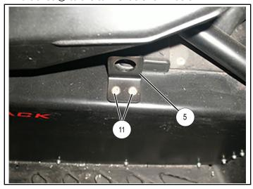
5. Place the new Fox air shock ② into position as shown below. Install new provided fasteners and torque to below specification. Route air filler hose as shown below.
