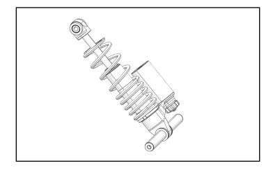
8. With the assembly removed, the shock can be removed from the cross shaft.
