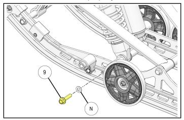
13. Using new hardware provided from kit, place new bushing ⓐ into upper shock rod ①. Place shock into skid for mounting. Place new screw ⑧ through shock rod mounting and torque arm bracket as shown below in assembly from left to right and tighten with nut ⑩.
