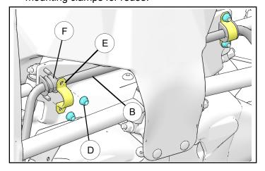
3. Remove sway bar (B) and bushings (F) from vehicle.
