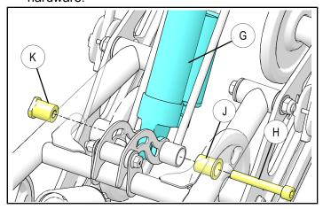
6. Install new shock assembly ⑤ onto lower mount using bushings ② ③ ④ and screw ⑦ as shown. Torque screw ⑦ to specification.
