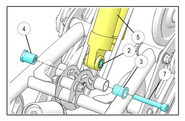
7. Install shock assembly ⑤ onto rear torque arm using bushing ①, screw ⑥, and nut ⑧ as shown. Torque screw ⑥ to specification.
