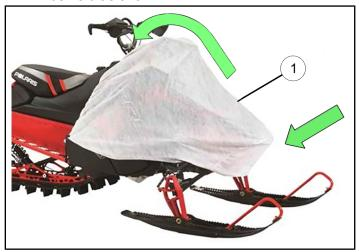
3. Use the side release buckle straps (A) sewn to the cover to secure undercover down. Feed the webbing strap down through the footwell (B) as shown and connect the buckles.
