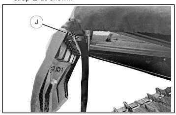
8. Lastly, adjust the front handle bar/windshield strap (k) (highlighted for clarity) to take up any excess material between the handlebars and windshield.
