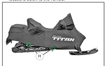
7. Move to the rear of the vehicle and secure the rear strap ① as shown.
