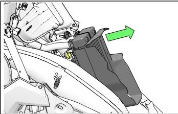
c. Once top is out of mount, pull up on radiator until it is disengaged from the lower mount.
