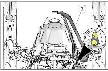
b. Place LH side tube ② into position as shown. Loosely install with provided M8 X 30 outer side tube fasteners ④ as shown.
