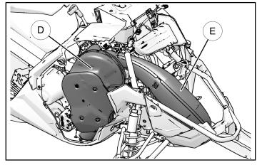
c. Remove remaining 4 exhaust springs securing exhaust pipe to chassis then remove exhaust pipe (E).
