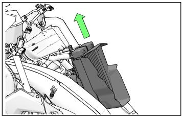
d. Carefully tie radiator to the side, out of the way, with a suitable strap.
