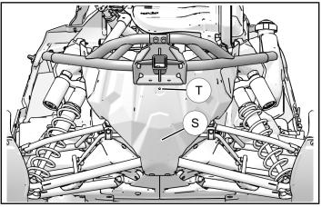
b. Remove the forward most A- arm mounting bolt (1) and nut (1) and discard.
