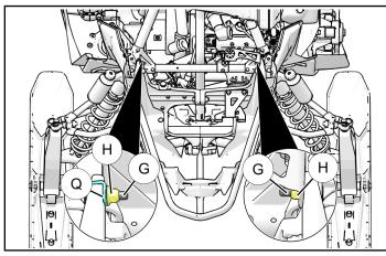
Remove the upper support bolt ①, lower support bolt (k) and locking nuts ① and remove bumper support (M).
