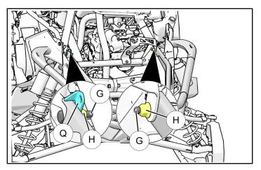
d. Reinstall the nose pan to side bumper screws
