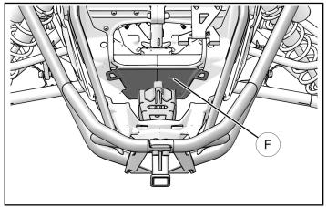
Once installed, place new piece of heat shielding material (1) into original location as shown.
