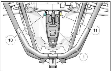
Next, reinstall original M6 lower support fastener ( and lock nut ( as shown.
