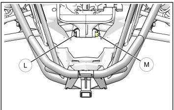
c. Place front bumper support ① into position. Insert provided M10 support bolt ⑩ through the bumper support and forward A-arm mounting hole. Loosely install locking nut ⑪.Next, reinstall original M6 lower support fastener and lock nut as shown.
