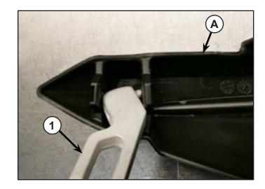
3. Pivot the mount so that that it falls naturally into the slot of the handquards. See figure.
