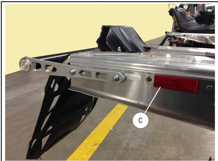
3. Install rear bumper ① using fasteners ② and ③. Install bolts ② with nuts ③ on outside of tunnel. Torque fasteners to below specification.
