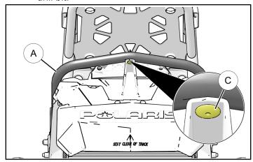
b. Next, remove four fasteners (B) holding the rear bumper (A) to the chassis and pull the bumper rearward and upward to remove.
