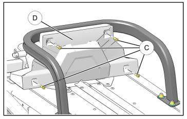
e. Torque the four main locking nuts 2 to the provided specification.
