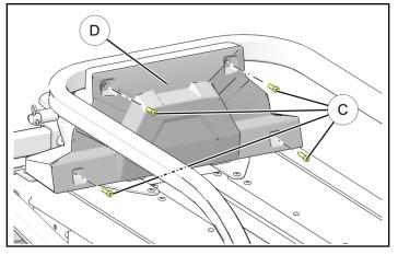
c. Next, remove the two rear most support fasteners  $\textcircled{\ensuremath{\mathbb E}}$  as shown.
