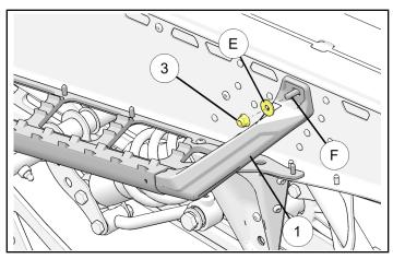
8. Repeat Step 1 through Step 7 for installing RH running board ②.
