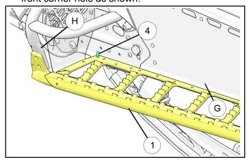
5. Using rivet gun install rivets ⑤ into running board ① holes in the bottom up vs top down orientation as shown.
