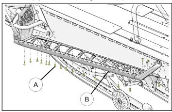
Using 10mm wrench remove nuts (D) and carriage bolts (C) from the front of running board (B). Discard nuts (D) and retain carriage bolts (C) for reinstallation.
