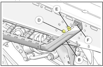
4. Align new LH running board ① mounting holes with LH side tunnel (G) and footrest (H) holes. Loosely install rivet ④ from bottom side into the front corner hole as shown.
