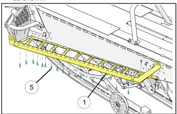
6. Install carriage bolts (C) and new nuts ③ attaching front of the running board ① to the footrest (H) as shown. Torque nuts to specification.
