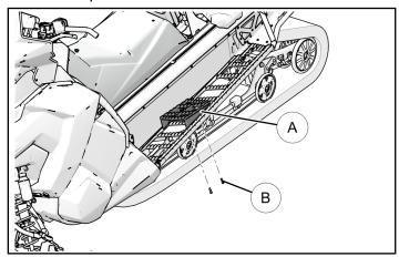
2. Place closeout panel ① on the underside of the running board and line up the mounting holes as shown.
