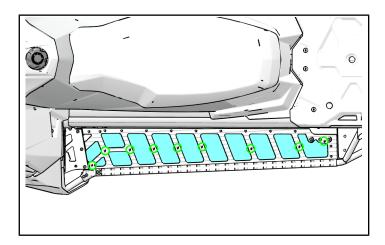
3. For vehicles equipped with passenger footrests, fasten the close out plate to the underside of the running board along with the footrest back into the original position using the provided screws ③ and washers ④ (two per side). If your vehicle does not have passenger footrests move on to step 4.
