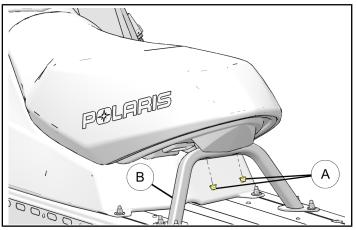
2. Pull up on rear of seat to disconnect from seat hoop.
