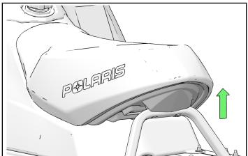
3. Install new kit supplied seat ① making sure that the front seat tab (D) mounted on the gas tank tab gets inserted into the slot (C) on the seat as shown.
