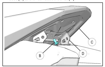
3. Pull back stock seat (C) so the front seat latch (F) disengages from locking feature (E) on the fuel tank as shown. Remove stock seat (C) from the vehicle.
