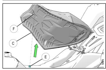
4. Install new seat ① onto vehicle making sure that the front seat latch (F) engages with the locking feature (E) on the fuel tank as shown.
