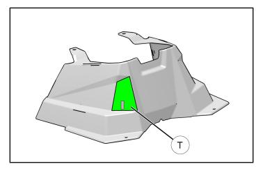
5. Install seat switch ② into slot by firmly pressing on switch face until completely seated.
