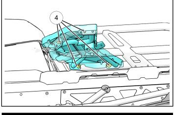
**TORQUE** 7.5 Ft. Lbs (10.5 Nm) 10. Install the passenger seat onto the vehicle by inserting the seat attachment hooks ① on the bottom of the seat into the two attachment slots (1) in the seat support making sure they fully engage the upper front portion of the cargo rack.
