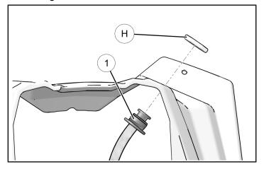
After installing harness plug, connect the white plastic female connector to the mating connector on the chassis harness as shown.
