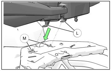
Once the front hooks (1) are engaged force the back of the seat assembly down until the latching pin (1) locks into the latching mechanism (2). Test to make sure the seat is fully secured by pulling on the hand holds and the seat back.
