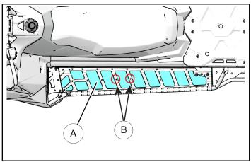
Place the passenger footrest ① on the running board, line up the mounting holes as shown with the holes that are indicated in the previous step for rivet removal and attach using the provided screws
