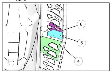
c. Carefully drill 7/32 inch (5.5 mm) hole at each marked location.
