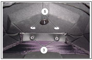
5. Insert Tuflock® rivet ④ in holes in rear of bag and fasten to rack.
