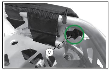
5. Secure lower front strap (1) into the location shown.
