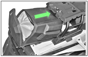
2. Once the bag is in position secure in place using the two indicated hook and loop fastener panels on each side of the bag. The hook and loop fastener panels should be wrapped tightly around each rear rack frame tube as shown.
