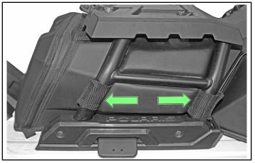
3. Ensure rear access zipper is closed and bag has been fully secured.
