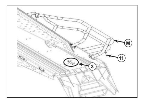
8. Mount deluxe rack on front side by attaching M6 nuts (11) and relevant washers (12) as shown.
