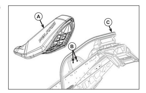
Remove four M6 nuts (B) and relevant washers (D) to remove weld support (C) and also remove four M6 bolts (E) by slide from tunnel panel.
