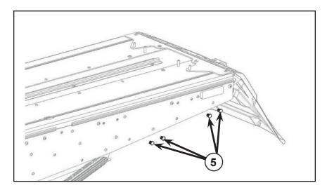
7. NOTE: First slide four M6 bolts in to the tunnel panel and adjust according to deluxe rack mounting.
