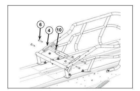
10. Install deluxe rack with taillight assembly (N) that was removed in step 3 and 4 using screws (8) and nuts (11) as shown in figure.
